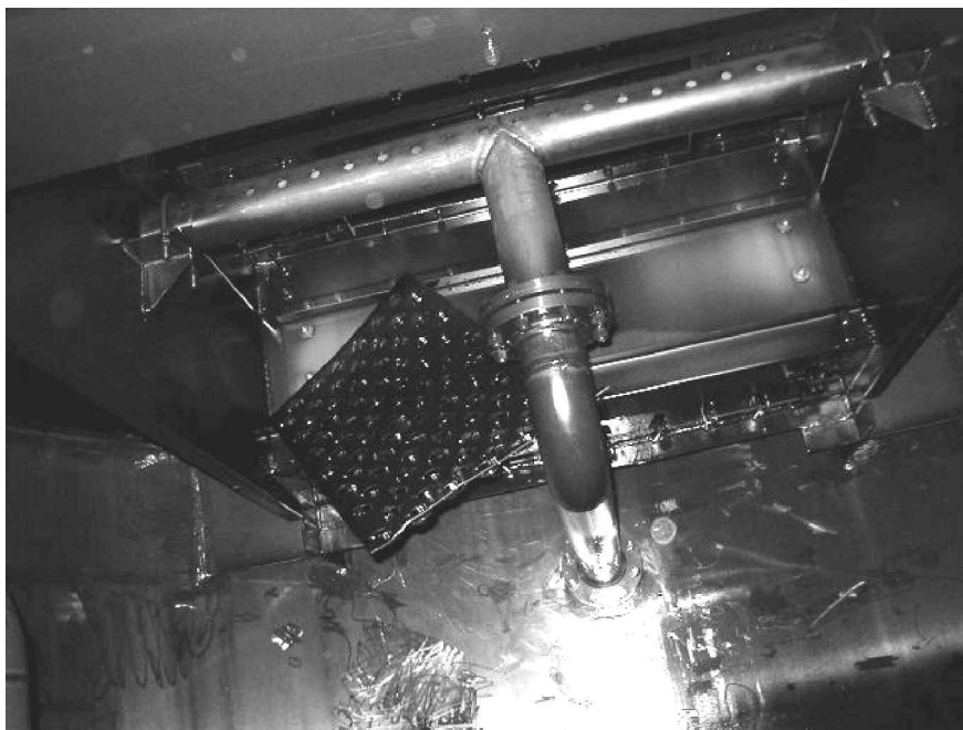
Figure 3. A displaced panel on the bottom tray in a refinery crude tower, the work of a water-induced pressure surge. Water-induced pressure surges can cause more severe damage; Amoco (1984a) has illustrations. The tower base is a common troublespot.
