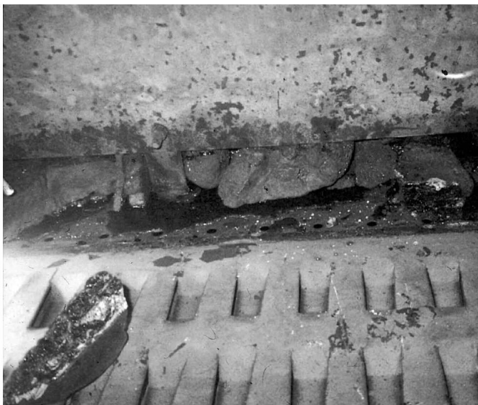
Figure 7. Incorrect assembly of tray panels is one of the most common assembly mishaps. Here panels of fixed valve trays were installed upside down. Also note the rocks in the downcomer; fouling was also a major issue in this tower. This diagram highlights the importance of inspecting tray and packing installation.
