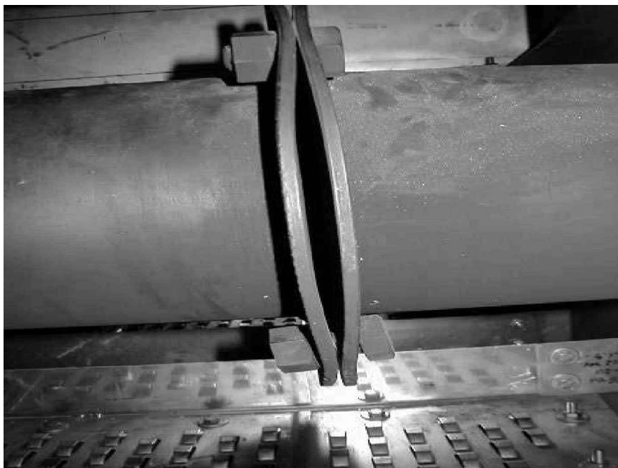
Figure 5. Damage often results from insufficient mechanical resistance. Flat-plate flanges on internal pipes, such as those leading to feed and reflux distributors, are weak and tend to spread apart. Gasketed raised face flanges of the appropriate pressure ratings should be used.
