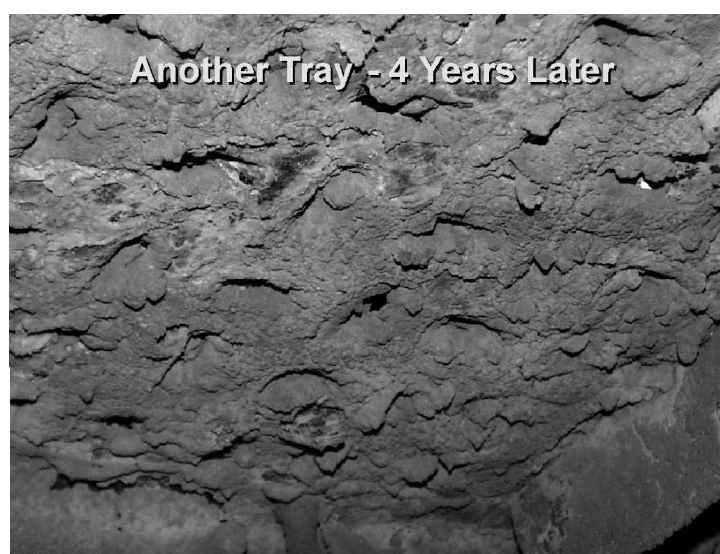
Figure 2. Even fouling-resistant trays are not immune to plugging under severe fouling conditions. These photos show active areas of one of the more fouling-resistant tray types in the industry plug up over a 4 year run. The plugging is believed to have been caused by severe salting out, a common cause of plugging.
